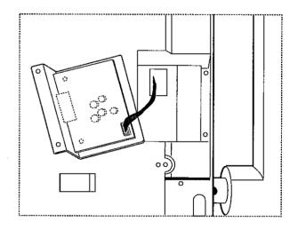
(3) Secure the RS-232C to the price computing scale with the screws provided.
